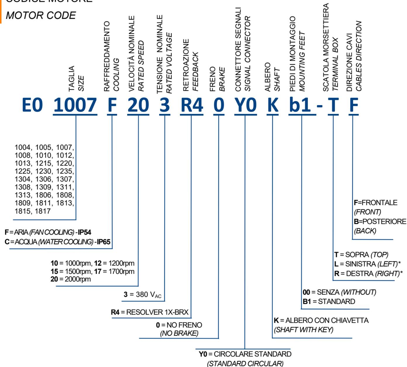
ESEMPIO D'ORDINE: **E0 1007 F 20 3 R4 0 Y0 K b1 - T F** = SERIE E0, TAGLIA 1007, VENTILAZIONE FORZATA, 2000rpm, 380V<sub>AC</sub>, RESOLVER, SENZA FRENO, CONNETTORE CIRCOLARE SEGNALI, ALBERO CON CHIAVETTA, PIEDI STANDARD, SCATOLA MORSETTIERA SOPRA, DIREZIONE CAVI FRONTALE.
